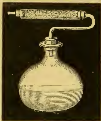
Apparatus for estimating the loss by weight of carbonic acid from fermentation.
